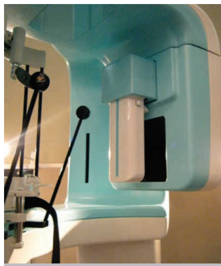
Figure 1 The Asahi Roentgen Alioth seen with a panoramic sensor mounted in front of the CBCT flat panel. This unit was shown at the Asian Congress on Oral and Maxillofacial Radiology, Nara, Japan, November 20-22, 2008.
